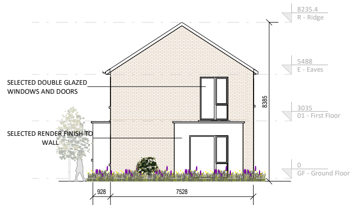
2 H07A Right Elevation (Brick) 1 : 200
